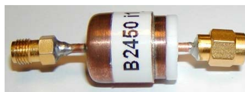
Figure 2 - RF Choke for measurements.
